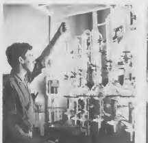
LEAD CONTENT in gasoline sample is measured in this test being performed by Loreto Kock, Tester A, a former LVS student.
